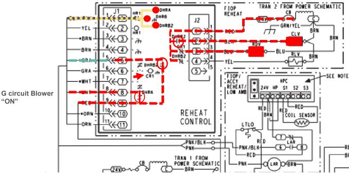
Tran 2 transformer powers the control circuit to Reheat contacts and solenoids.
