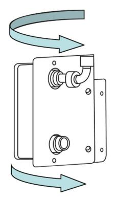
Rotate 90° (<sup>1</sup>/<sub>4</sub>-turn) to align parallel to filters.
