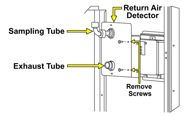
As received in the field, the components are mounted together.
