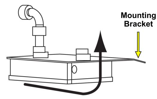
Rotate the return air detector end-to-end to where the elbow fitting is pointed down. Notice the mounting bracket has a slight bend to it.
