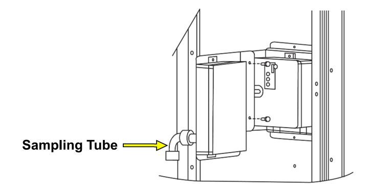
Attach return air detector to controller using mounting bracket.
