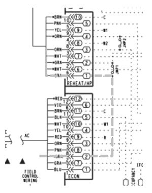
When HumidiMiZer Reheat board is added to a system. Jumper 1, 2 & 3 will be cut and removed.
