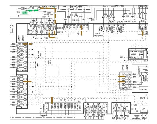
24v common is any of the brown wires in control panel on any control board or component
