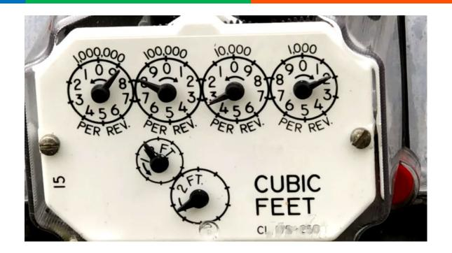
We clocked the meter, and it takes 62 seconds to consume 1 cubic foot of gas
