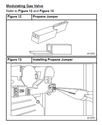
NOTE: The Propane jumper for the modulating gas valve is very small. Needle-nose pliers are required to insert the jumper into the valve. If the jumper is not installed, the valve will not operate properly on propane.
