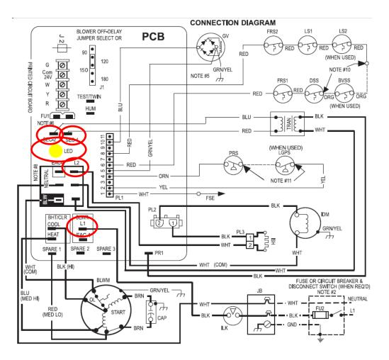
If Status Light is on continuously, furnace is powered, and board has 24 VAC power
