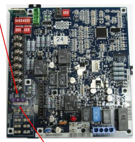
Automotive-type Fuse All furnaces have low voltage fuses on their boards.
