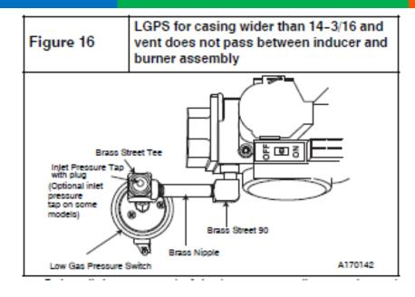
Always check gas pressure both supply and manifold
