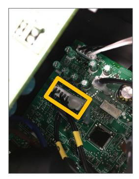
Take T2B - T2 temperature = superheat of the Evaporator. On average around 7SH
